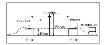
We measured the loudness of the sound passing through Barrier A ten times, when x=37.5cm. We also performed the same experiment for when x=75cm, 150cm, and 300cm, and this operation was repeated five times. The average value calculated by this measurement was regarded as average (A). We performed the same experiment for Barrier B and Barrier C, and the average (B), average (C) were calculated.
