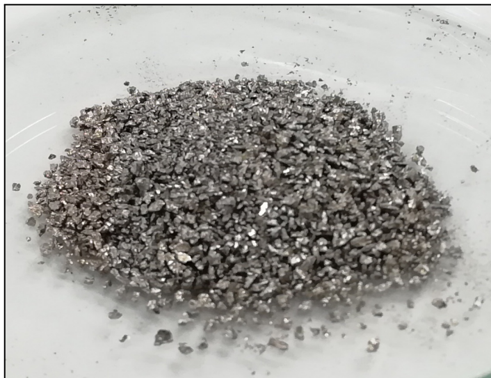
Fig.2 CaNi 5 , one of the MH Alloy
